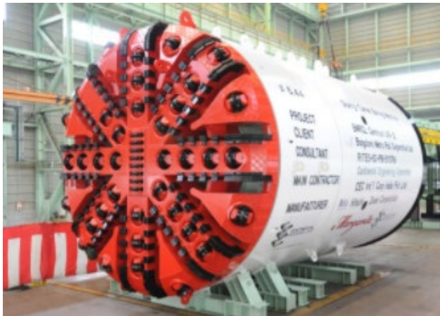
Closed face TBM
